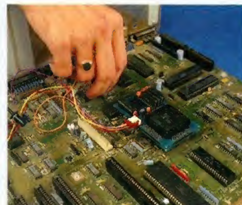
7 Attach the crocodile leads very carefully. They must be attached to the correct pins and they must not short out the legs of the Gary chip.
